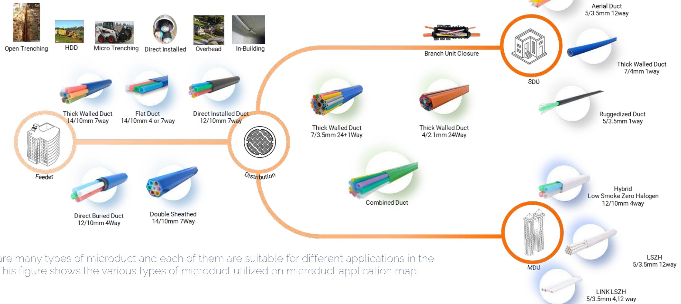
Here are many types of microduct and each of them are suitable for different applications in the field. This figure shows the various types of microduct utilized on microduct application map.
